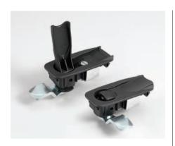
The composite Lift & Turn latch is a light- to medium-duty latch, utilizing engineering plastic in its major components to reduce weight yet maintain excellent strength. When the lever is in the upright position, it rotates 360° to move the cam behind the support in any one of three 90° positions. Once in place, the lever closes flush with the housing, providing 5 mm of axial pull, locking the device with an over-center action.
