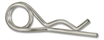
A double loop adds flexibility for a wider fit range of this Cotter Pin, compared to R Clips or other Cotter Pin Clips. Stresses are evenly spread throughout the loop, giving longer life and more repeatability. High quality part made of hard drawn MB spring wire, zinc plated and baked.
