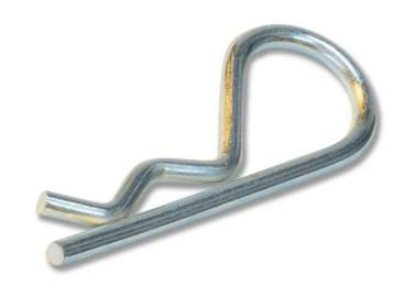
Hair Pin Cotters (or "R Clips") are a spring-type cotter made to be reusable. Hair Pin Cotters are generally meant to be used in through-holes while Hair Pin Clips are generally meant to be used on a groove. Double Loop Hair Pin Cotters are also available.
