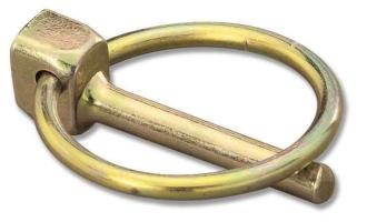
plated zinc with a yellow chromate dip for added corrosion protection. Steel Lanyards or Nylon Lanyards may be added as a low cost tether to prevent Lynch Pin loss. These quick locking pins do not require cotter pins and are faster to use than clevis pins and cotters.
