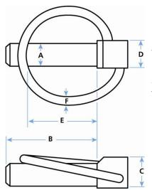
The ring is made from hard drawn MB spring wire.
