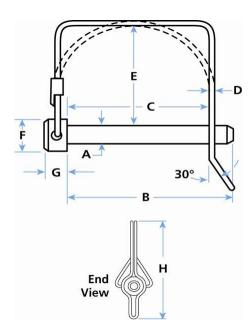
Steel Lanyards or Nylon Lanyards may be added as a low cost tether to prevent loss. These quick locking pins do not require cotter pins and are faster to use than clevis pins and cotters.
