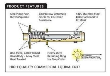
Ball Lock Pins are a very secure quick-release pin. They have a push button that initiates ball action and retraction, and can only be released by pushing the button. Ball Lock Pin design combines secure fastening with Quick-Release ease of removal. Steel Lanyards or Nylon Lanyards may be added as a low cost tether to prevent loss
