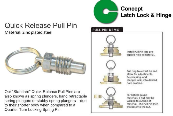
The Quick-Release Pull Pin body is threaded into the application, with ring on outside surface. Pull the ring to retract spring-loaded tip and allow adjustments. Release the ring to lock Pull Pin tip into desired hole location. Chamfered tip allows for easy alignment. Spring Plungers are ideal for adjustable tubing, tooling, latches, fixtures, gates, and much more. Steel Lanyards or Nylon Lanyards may be added to the Spring Plunger ring as a low cost "pull actuator".
