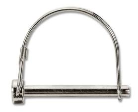
pin, Wire Lock Pins eliminate cotter pin loss and fit most Quick-Release applications. Steel Lanyards or Nylon Lanyards may be added as a lowcost tether to prevent loss. These quick locking pins do not require cotter pins and are faster to use than clevis pins and cotters.
