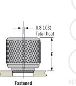
**Notes:** For use in material hardnesses RB85 or less, such as low carbon steels that are half hard or softer, stainless steels in the annealed condition and aluminum.
