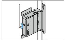
Closing speed is adjustable with a hex key. (size: 2.5)
